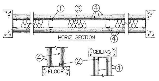
1. **Studs** — - Channel-shaped, min 1-5/8 in. wide by 1 1/4 in. deep, with 5/16 in. folded back return flange legs. Fabricated from No. 25 MSG galv steel. Stud spacing 16 or 24 in. OC. Studs to be cut 1 in. less than assembly height.
